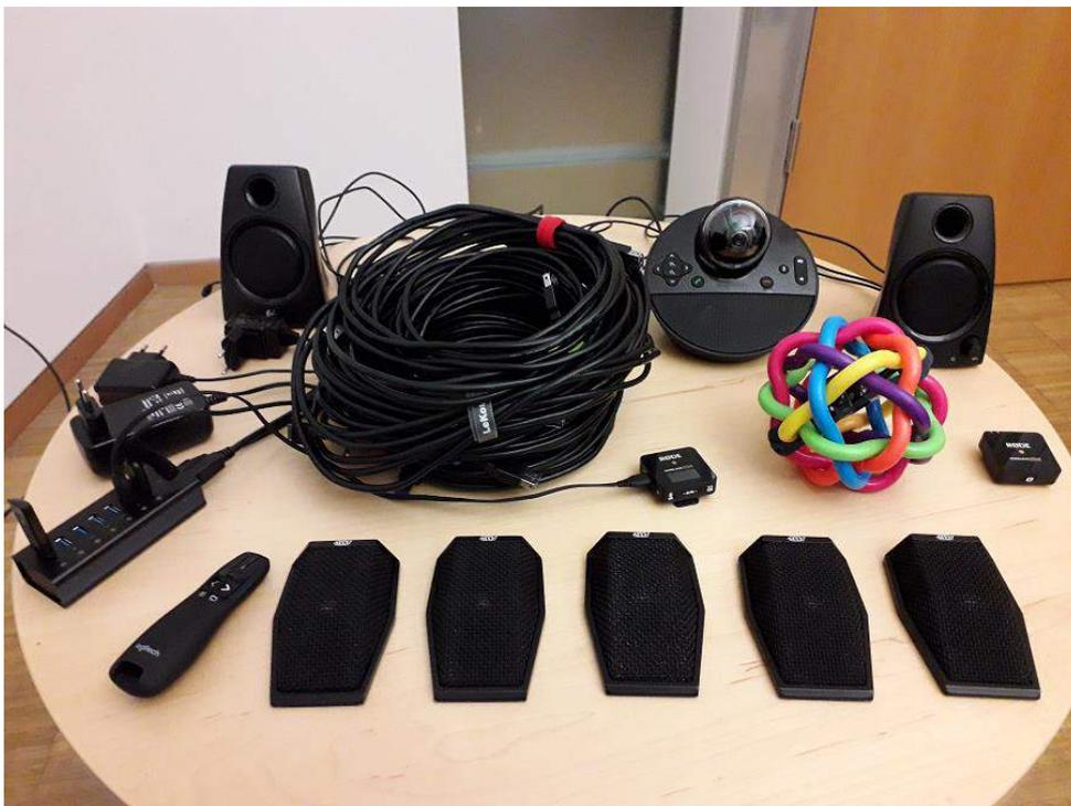
**Figure 5:** Components of the full setup. Next to the equipment shown in fig. 3, the full toolbox involves a number of MXL AC-404 or MXL AC-44 (here: five, front row) and the connecting USB cables and USB extensions (big pile in the center). Instead of the Logitech device and the external speakers, the Obsbot Tiny Webcam and the lecture theatre's speakers can be used if available (Fig. 6).
