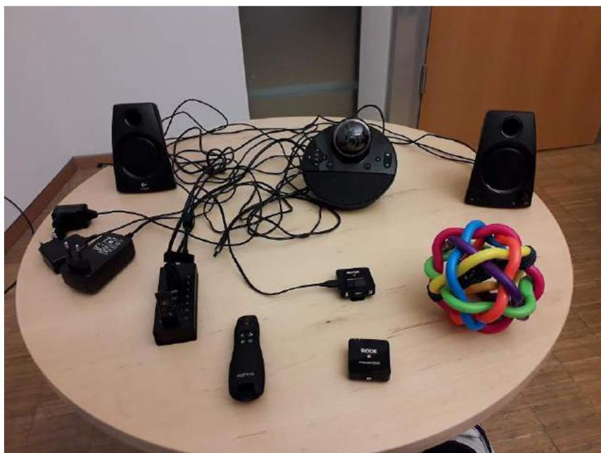
**Figure 3:** Components of the setup, with speakers and camera in the background, the Rode wireless microphones and receiver to the right, the presenter in the front, and the USB port extender to the left. Here, the audio signal for the speakers comes from the 3.5 mm jack of the laptop (select Windows Realtek audio driver).
