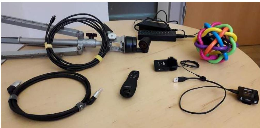
**Figure 4:** Components of the setup for large lecture theatres and blackboard writing. It features the Obsbot camera plus tripod and cable (lying, left), the throw-around and the Lavalier mic plus receiver (right), the port expander (background), an optional slide advancer (center), and the HDMI cable for video and audio output to the lecture hall theatre's installed equipment (left, foreground).
