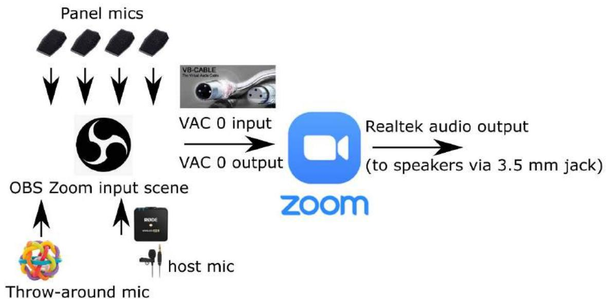
**Figure 10:** Setup (hardware and sound settings) for application 3: Mix a number of desktop microphones together with the wireless throw-around microphone (plus additional host microphone).
