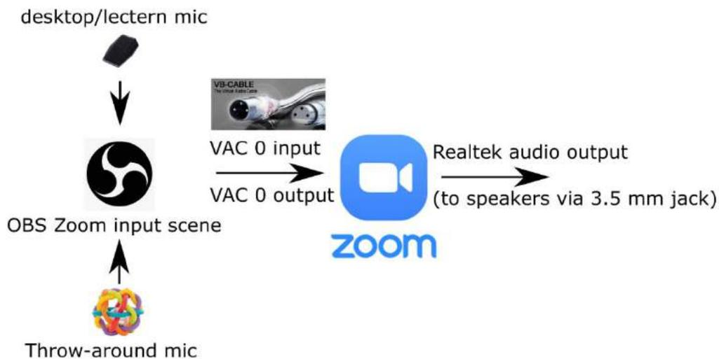
**Figure 8:** Setup (hardware and sound settings) for application 1: Mix one desktop microphone together with the wireless throw-around microphone.
