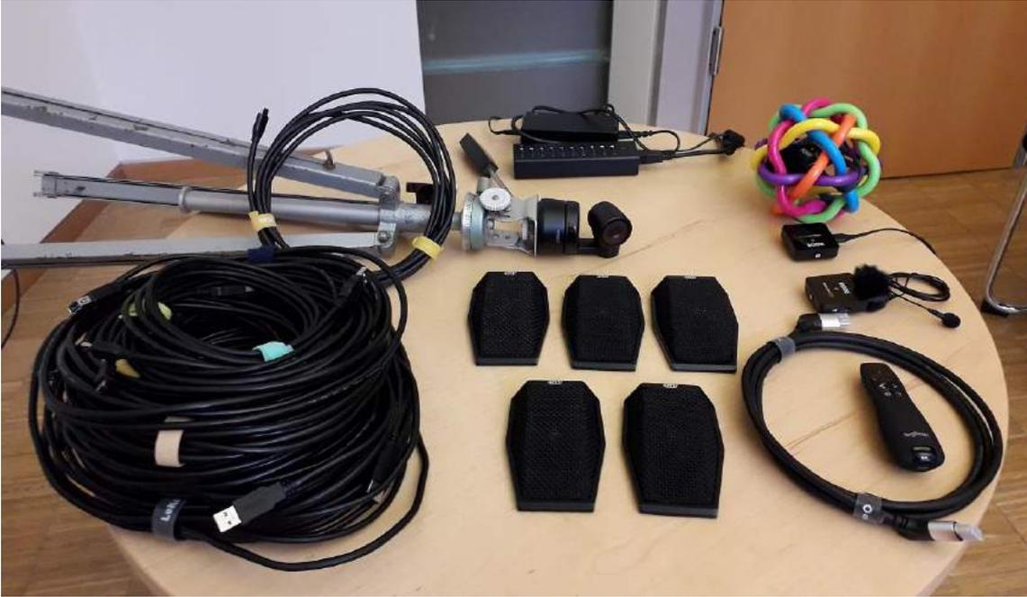
**Figure 6:** Components of the full setup, alternative to Fig. 5. Next to the equipment shown in fig. 4, the full toolbox involves a number of MXL AC-404 or MXL AC-44 (here: five, center) and the connecting USB cables and USB extensions (big pile, foreground, left). The Zoom audio output is send to the lecture theatre’s speakers via the HDMI cable (right).
